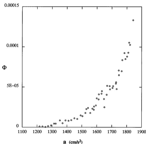
FIG. 2. Droplet rate data from  $\nu = 5$  cS Silicone Oil at 45 Hz: Each point represents the number of droplets (scaled with measurement parameters) produced in a 300 s period.
