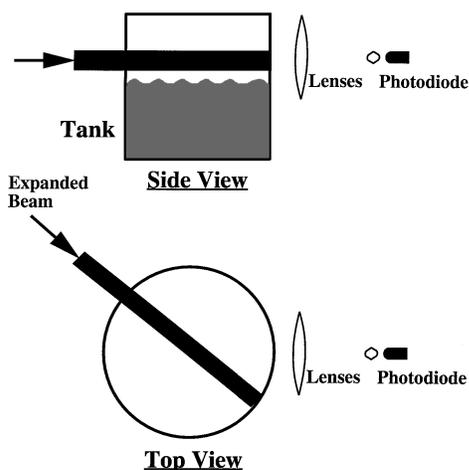
FIG. 1. A diagram of the experimental apparatus: The laser is directed at a  $40^\circ$  angle to the photodiode in order to maximize the signal from the ejected droplets while avoiding direct illumination and wall scatter.
