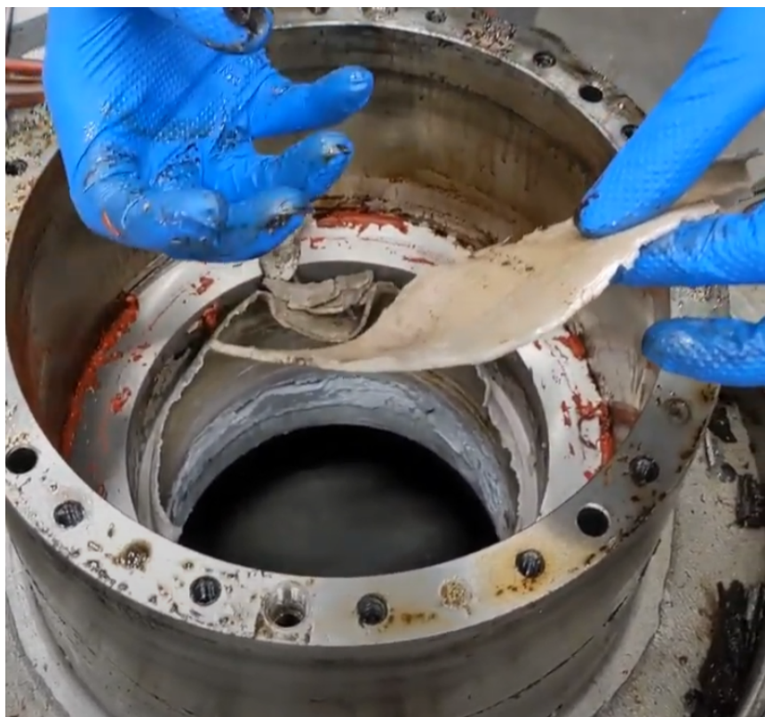
Figure 3.21: Rubén demonstrating pieces of sodium metal found in the different parts of the experiment during the cleaning operations.
