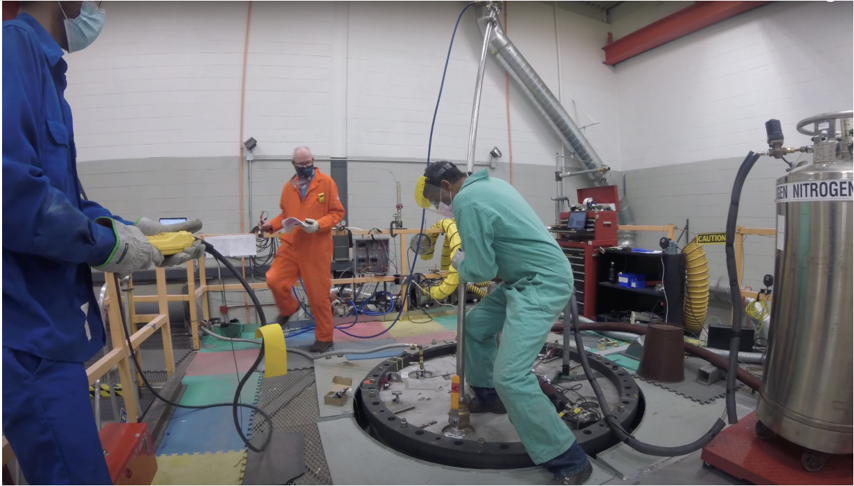
Figure 3.15: The insertion procedure: Rubén Rojas (in blue on the left) adjusts the height of the diptube with the overhead crane, Nolan Ballew (in green in the center) pushes the dip tube into the port with the valve and lip seal, and Dan Lathrop (in orange) checks the procedure protocols. The liquid nitrogen dewar is on the right and ready to be used in case of fire.
