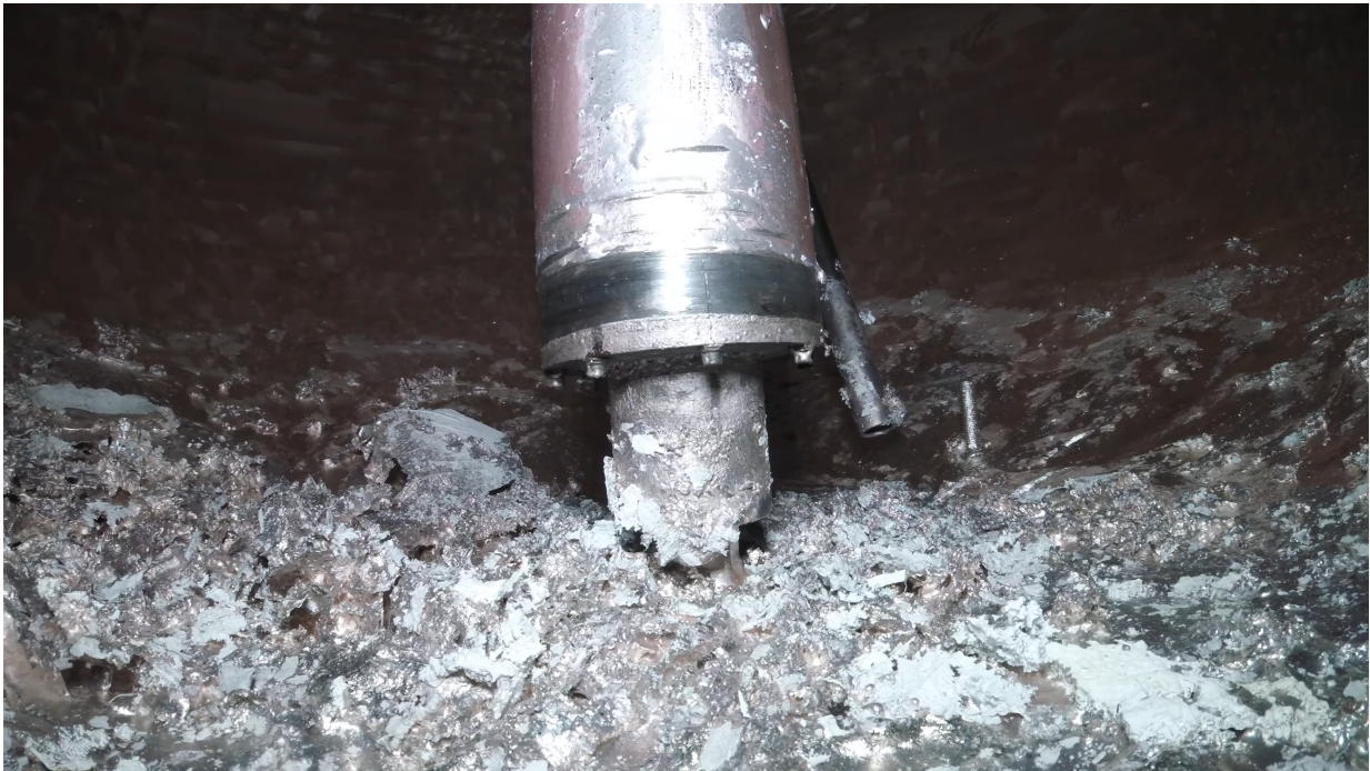
Figure 3.18: The picture from a GoPro camera inserted into the sphere after the sodium removal. The inner shaft is in the center of the image, and the bright textured debris at the bottom is sodium metal.
