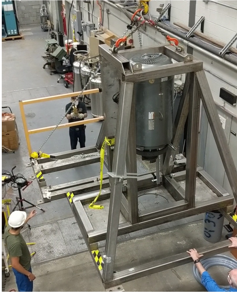
Figure 3.30: The rigging configuration for the inner frame. Two chain hoists allow controlling pitch and roll, while Dan's hands control yaw (bottom right).
