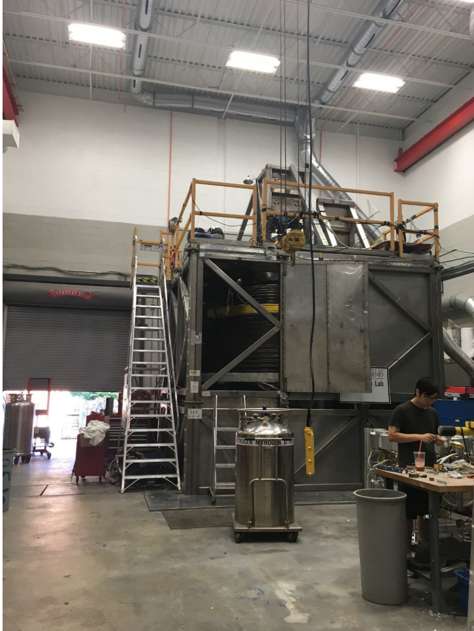
Figure 1.4: Photo of Three-Meter Dynamo experiment, the outer sphere is visible through the cube door in the center of the picture, the rolling door (on the left) was one of the main designing constrains, because one cannot fit a sphere wider than the opening.
