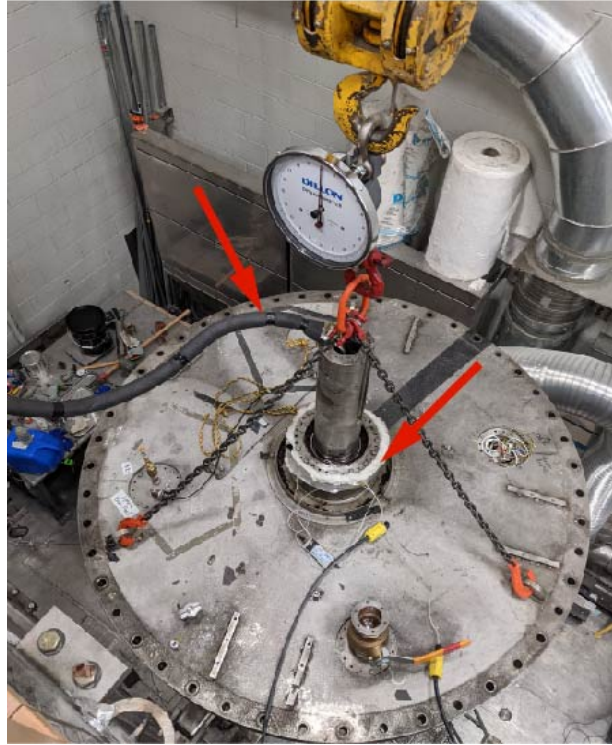
Figure 3.20: The decoupling process required applying liquid nitrogen to the shaft (the left arrow), and heating the bearing with the electrical tape (the right arrow).
