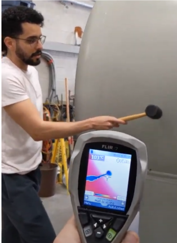
Figure 3.24: Liquid to solid ratio diagnostics in process. Rubén uses a mallet to bounce the surface of the tank, and the produced sound distinguishes the state of the matter inside. Also, the infrared camera shows different surface temperatures for different sounding regions.
