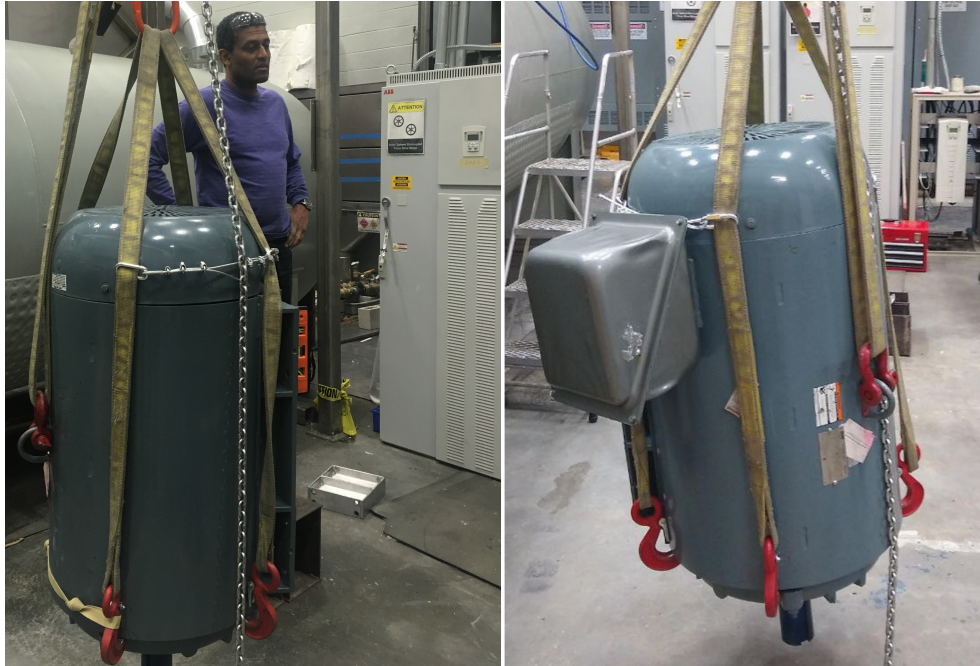
Figure 3.29: Rigging the outer sphere motor with multiple straps secured with cables, and a chain hoist that allows it to slip the motor before landing.
