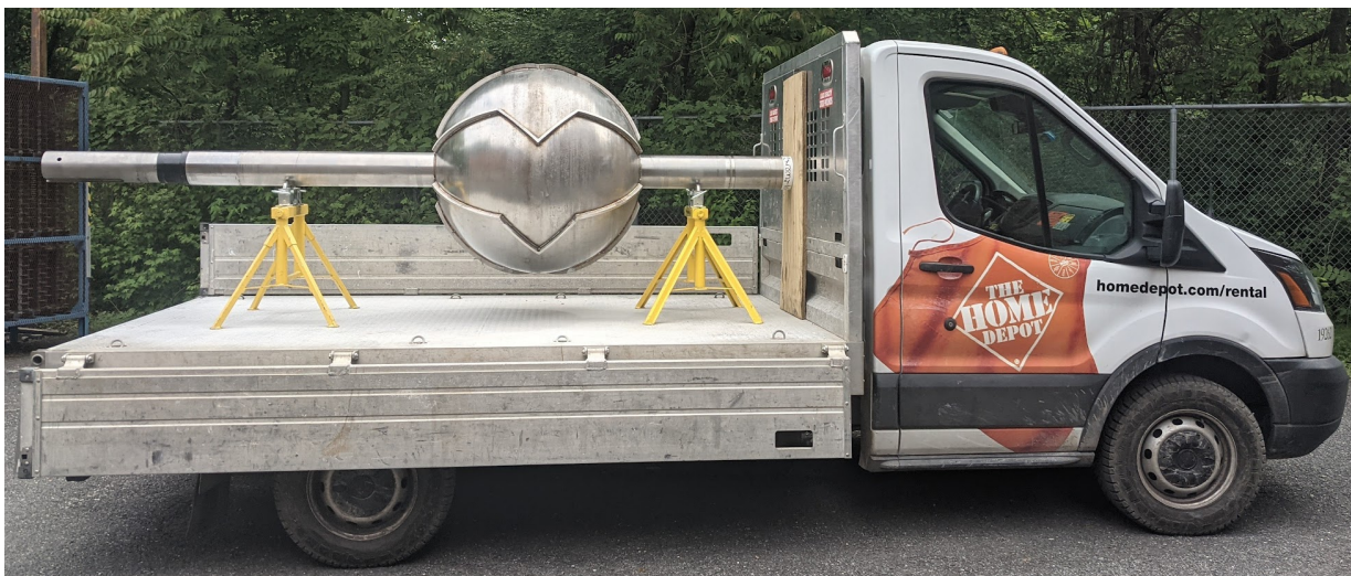
Figure 3.22: The new inner sphere on the day of delivery back to the lab. The black part of the shaft on the left is the thread covered with duct tape. During the unload we dropped the sphere on the ground from 40 cm height but that was nothing but a scratch.
