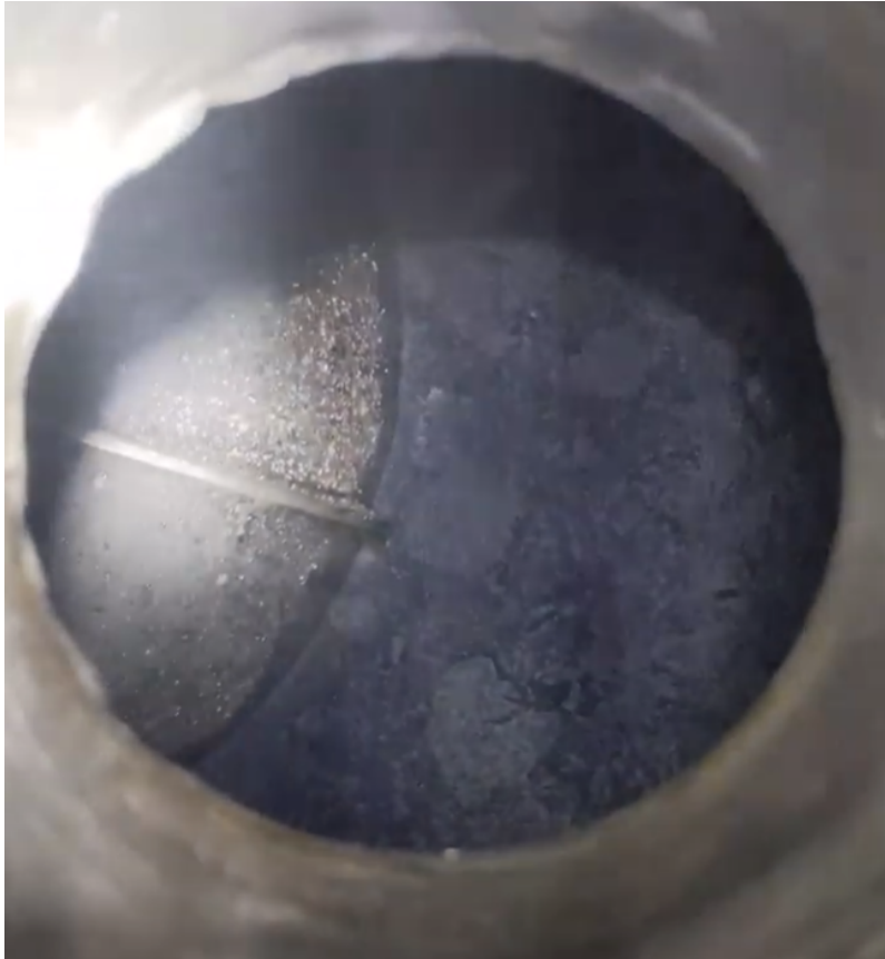
Figure 3.28: A photo of liquid sodium through the window port, filling up the sphere during the refilling operation.
