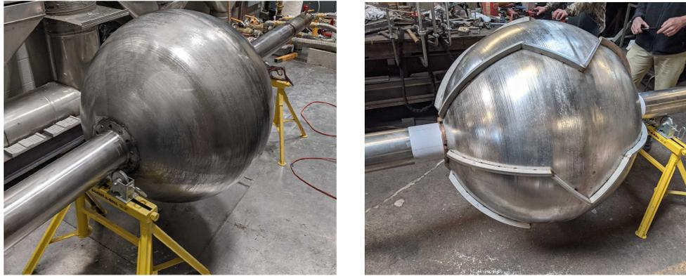
Figure 4.16: Left: Smooth inner sphere. Right: Rough inner sphere with alpha baffles installed.
