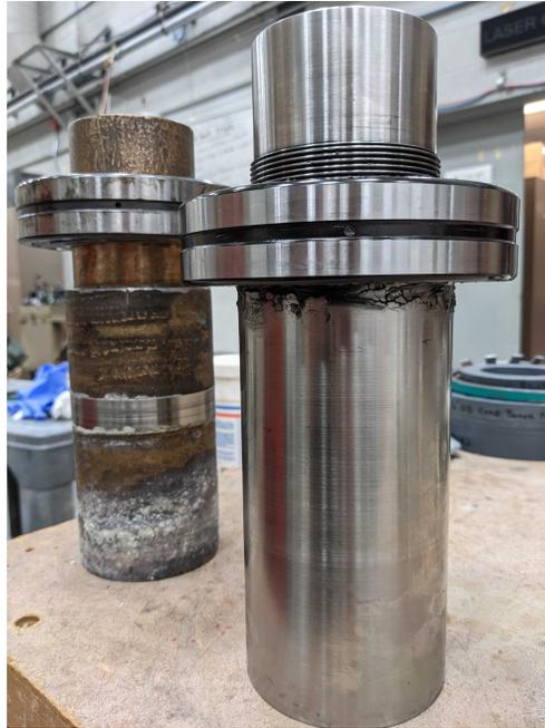
Figure 4.15: Left: Bottom view of the inner bottom bearing and the bayonet coupler after the bearing retainer and lip seals were removed. The dirty bearing can be spotted. Right: the new stainless steel bayonet coupler (front) and the old one (back), oiled infused brass alloy. A layer of oxide (white color) can still be seen after many wet cleans.
