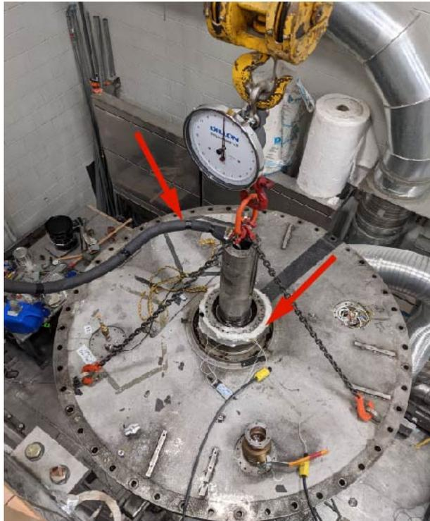
Figure 4.14: Installation used to release the top inner bearing from the shaft. Left arrow points at the liquid nitrogen hose pouring liquid inside the shaft aperture. Right arrow points at the heat tape used to heat up the bearing.
