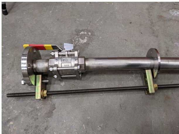
Figure 4.8: Spacer to support the dip tube and transfer line.
