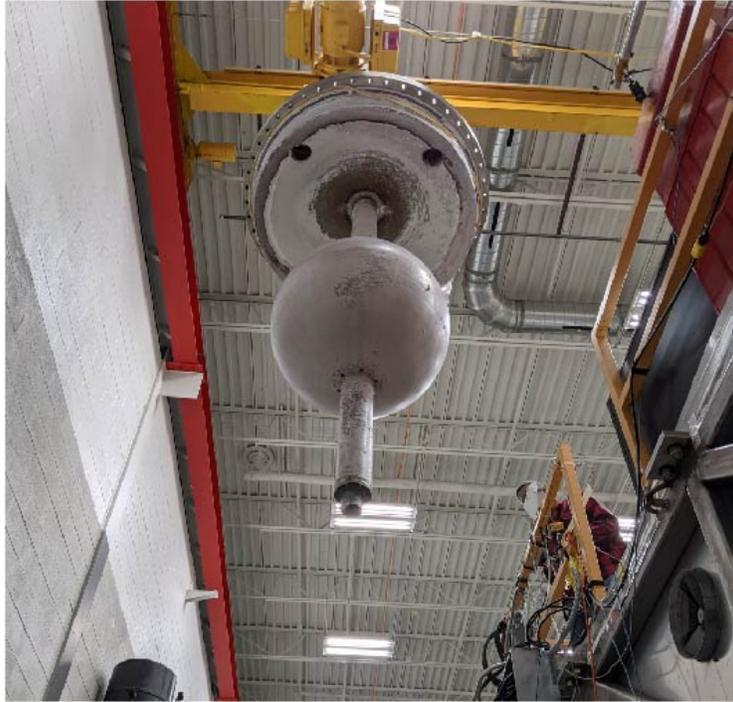
Figure 4.13: Flying inner sphere-shaft-lid combo. In the picture you can see the pink sodium covering the combo.
