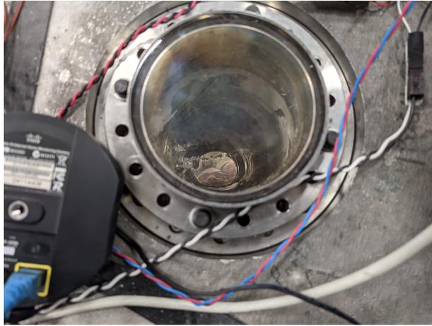
Figure 4.12: Visualization window on one of the ports of the experiment. Liquid sodium can be spotted from the window.
