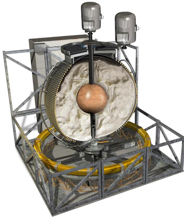
Figure 3.6: Rendering of the 3 m Experiment. The inner sphere and the outer spherical shell can be driven independently by their two respective motors (top). Liquid sodium serves as the working fluid for hydromagnetic experiments. Figure credit: Laurent Hindryckx.
