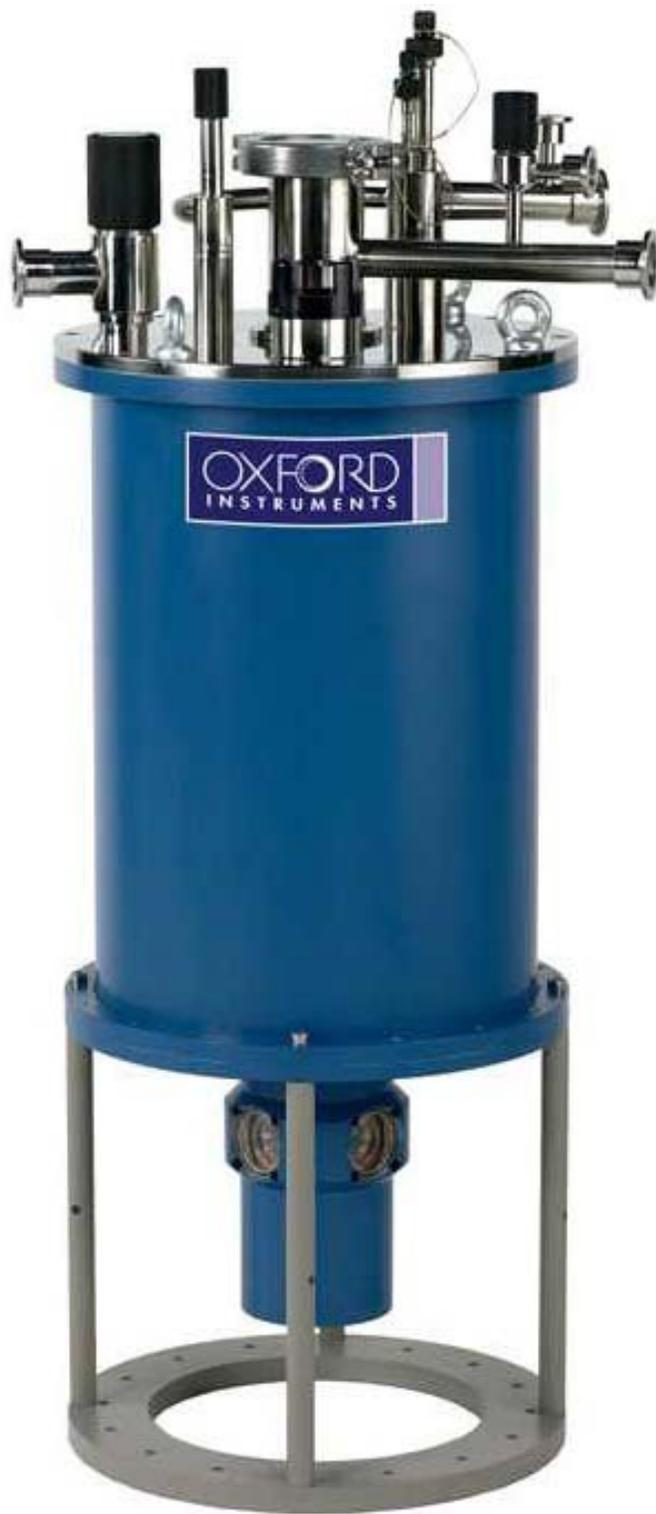
Figure 3.2: Photograph of the Oxford Instruments Optistat-SXM cryostat used in the experiments presented here.
