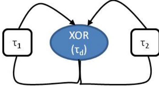
Figure 4.1: Example of Boolean Chaos. Two delays ( $\tau_1$  and  $\tau_2$ ) are inputs of XOR with response time ( $\tau_d$ ).
