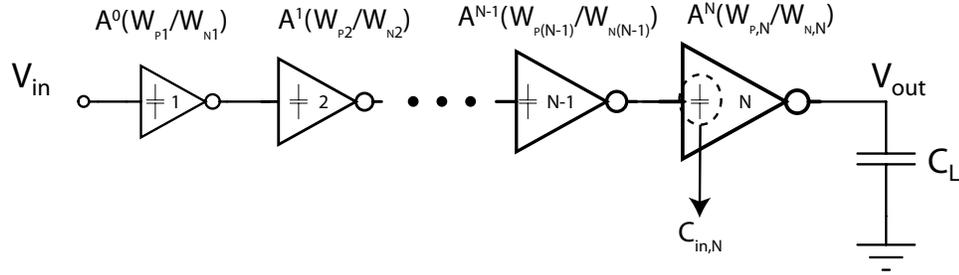
Figure 2.6: Schematic diagram of a cascaded scale-up buffer. The number of stages  $N$  should be an even number, and  $A$  is a scale ratio for the widths of transistors
