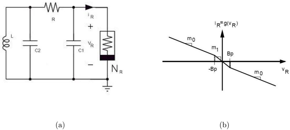
Figure 1.2: (a) Circuit diagram of Chua chaotic circuit. (b) Current-voltage transfer characteristics of Chua diode [19].
