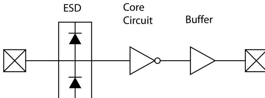
Figure 2.2: Basic components of CMOS digital circuit, consisting of electrostatic discharging (ESD) protection circuit, core circuit, and output buffer.
