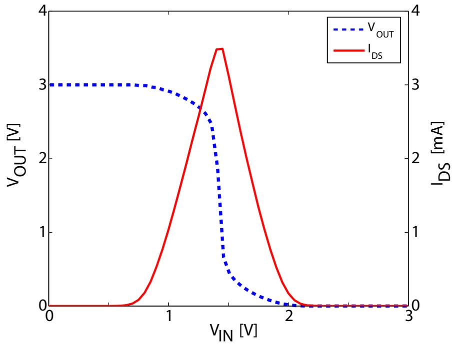
Figure 2.5: Experimental results of DC transfer characteristics and short current of CMOS inverter in DC condition. Peak current of 3.5 mA is measured when DC input voltage is at 1.5 V.
