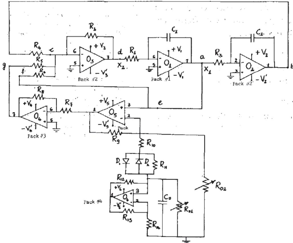
Figure 1.3: Circuit diagram of an RC Op-Amp chaos generator using a hysteresis [21].
