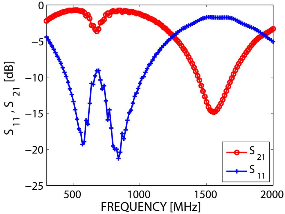
Figure 3.4: Forward transmission coefficient  $S_{21}$  (red) and forward reflection coefficient  $S_{11}$  (blue). Notice there is a 4dB decrease in  $S_{21}$ , meaning less than half of input power is transmitted at the frequency around 700 MHz.
