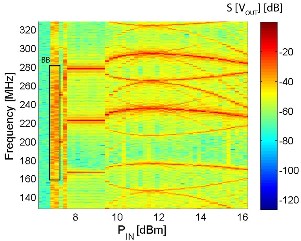
Figure 2.13: Evidence of chaotic oscillation such as complex spectrum and broadband spectrum (BB).
