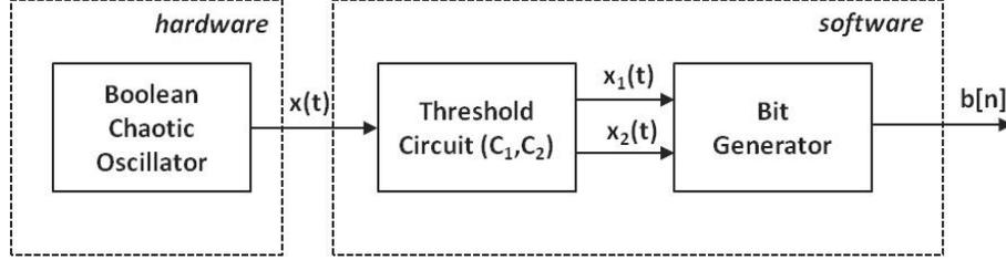
Figure 5.1: Schematic diagram of random number generation using CMOS boolean chaotic oscillator.
