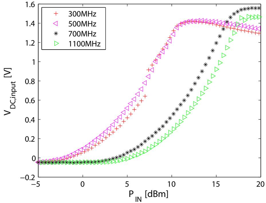
Figure 2.15: Experimental results of rectified DC input voltage (time-average values). Input voltage is measured across a large resistance connected at the bias tee. Input voltage is rectified at 1.4 V due to the rectification of ESD diodes, resulting in a DC offset at the circuit input.
