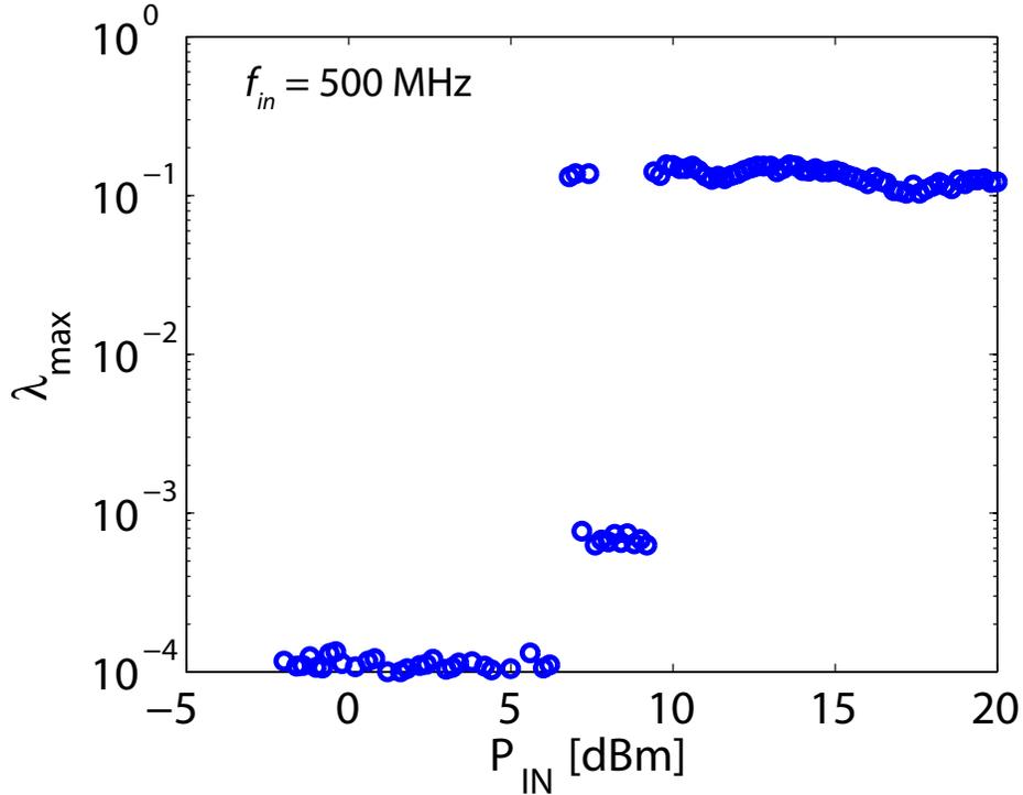
Figure 2.14: Largest Lyapunov exponents ( $\lambda_{max}$ ) with varying  $P_{IN}$ . The measured data for each  $P_{IN}$  are calculated for  $\lambda_{max}$ . The circuit is driven with input RF signal with a frequency of 500 MHz, as in Fig. 2.12(b).
