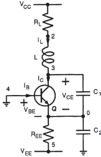
Figure 1.5: Circuit diagram of a bipolar junction transistor Colpitts oscillator [24].
