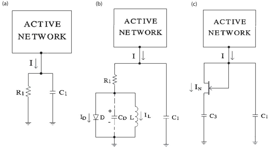
Figure 1.7: Classes of core chaotic oscillators. (a) sinusoidal oscillator with a parallel RC, (b) using diode inductor composite, and (c) with FET and capacitor composite [33].
