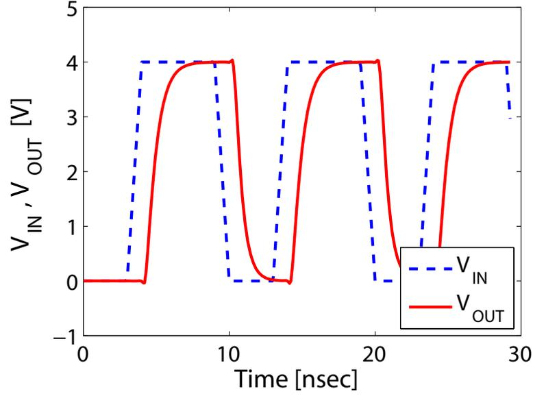
Figure 2.7: Time evolution of input and output voltage of the designed buffer. The simulated results show that the output of buffer has only a small time delay.
