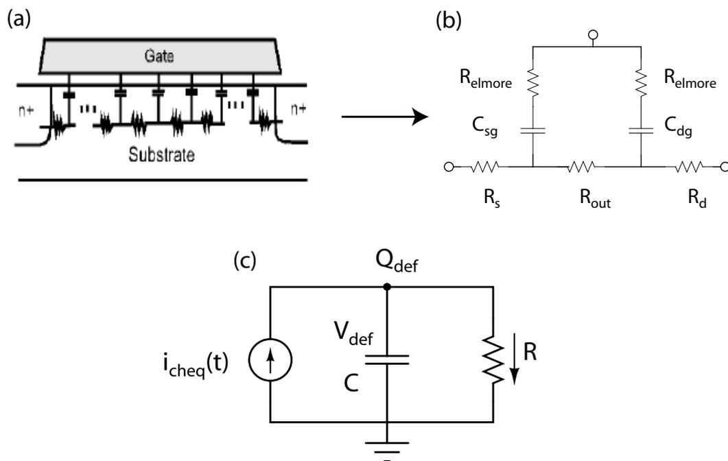
Figure 3.1: (a) Diagram of charge-deficit Non-Quasi-Static model. (b) Diagram shows an equivalent network for the channel of MOSFET. (c) NQS sub-circuit for transient analysis.
