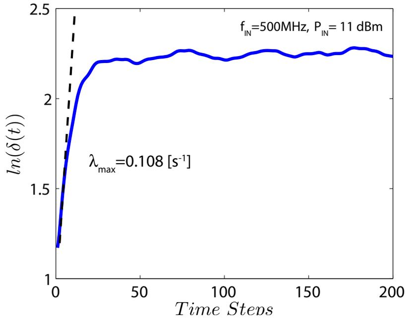
Figure 3.12: Average logarithmic distance between trajectories corresponding to Fig. 3.10(b). The initial positive slope (the positive largest Lyapunov exponent) and a long time saturation of the average distance indicate chaotic dynamics.
