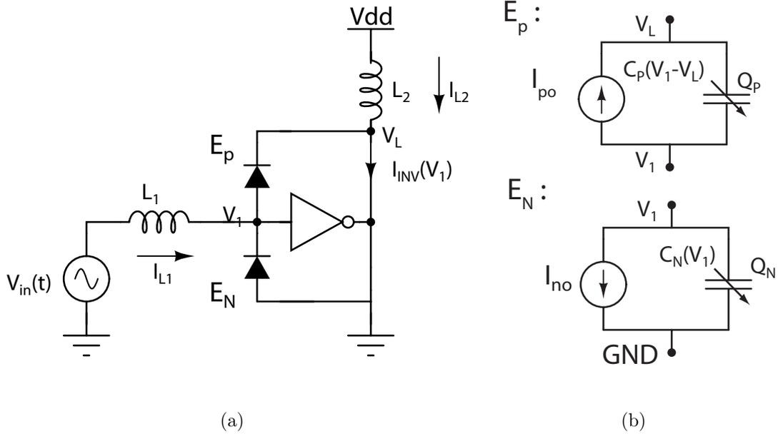
Figure 3.8: (a) Simplified circuit diagram of a CMOS inverter coupled with ESD circuits for numerical modeling.  $L_{1,2}$  is an equivalent parasitic impedance around 5 nH. (b) Dynamics of ESD protection circuit for gcPMOS and ggNMOS.
