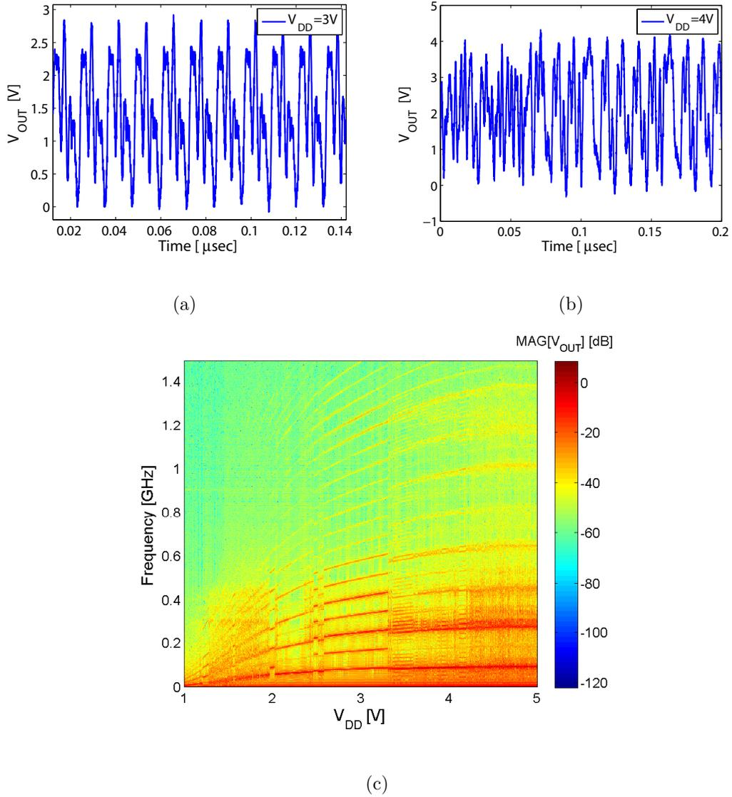
Figure 4.4: (a) Time evolution of periodic oscillations when the circuit is biased at 3V. (b) Time evolution of chaotic oscillations when the circuit is biased at 4V. (c) Frequency spectrum of output voltage signal with varying  $V_{DD}$ . A broad spectrum with numerous subharmonics is observed, reaching from DC to 500 MHz.
