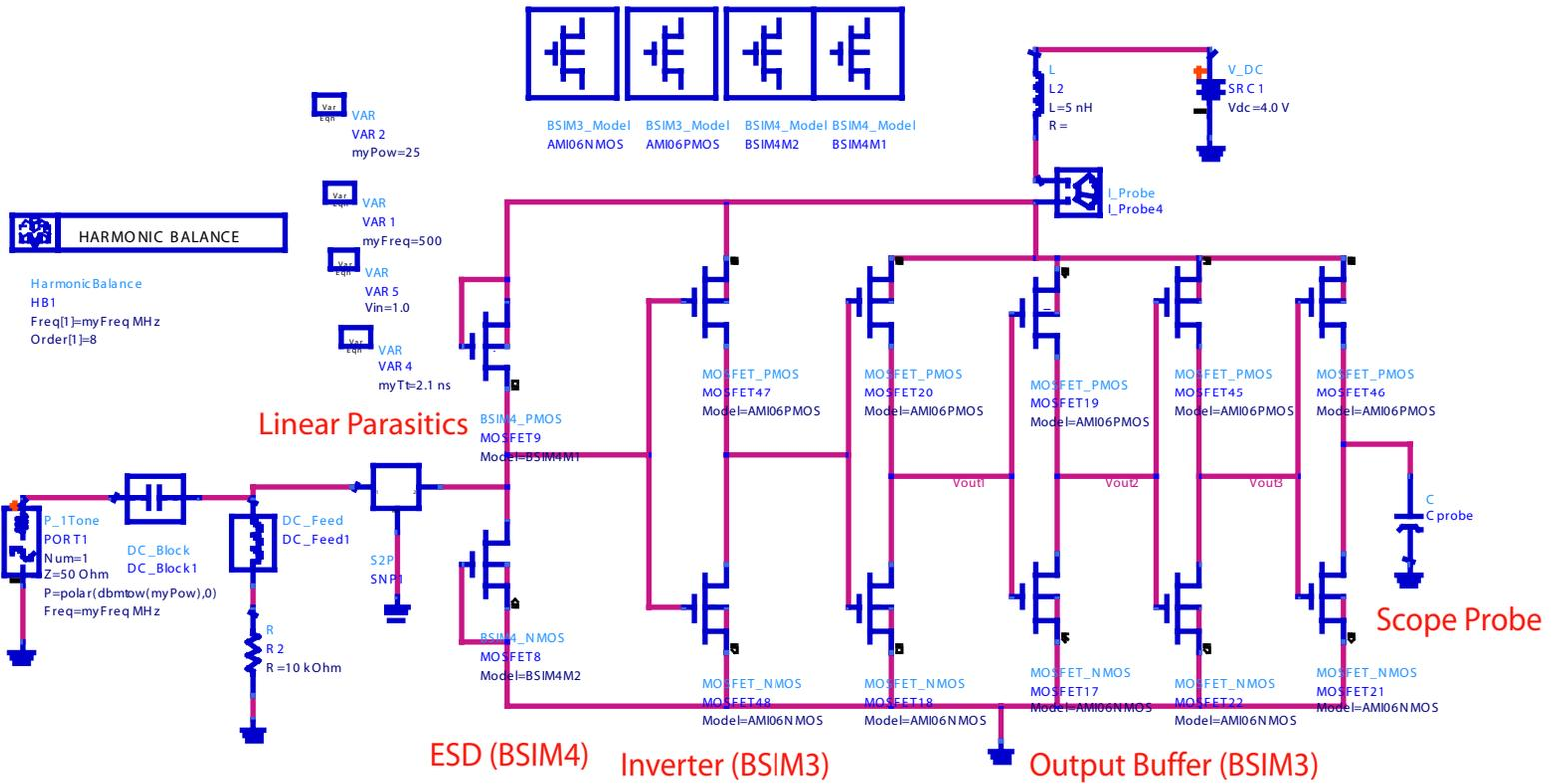
Figure 3.6: A complete schematic created with ADS software. The BSIM 4 model is included as well as the input parasitic model. The BSIM SPICE parameters are extracted from test results provided from the foundry.
