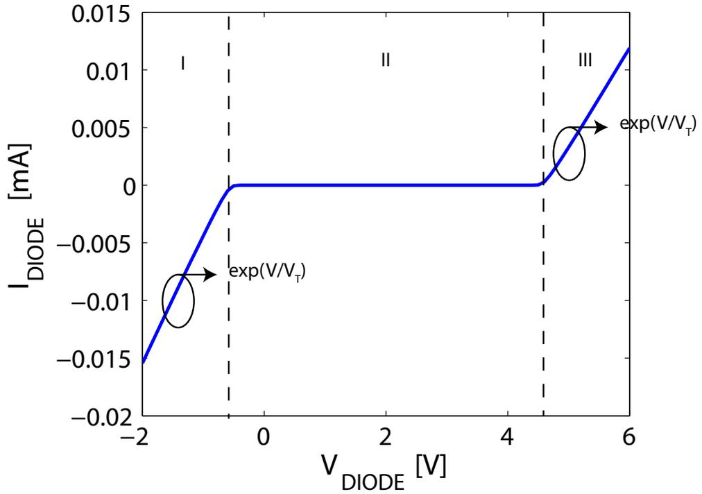
Figure 2.9: Simulation results of current-voltage characteristics in our ESD protection circuits. In Region I, ggNMOS turns on, and gcPMOS turns on in Region III, and finally ggMNOS and gcPMOS remain turned off in Region II. The circuit is biased at the supply voltage of 4V. Current-voltage transfer curves in Region I and III follows the Shockley diode equations.
