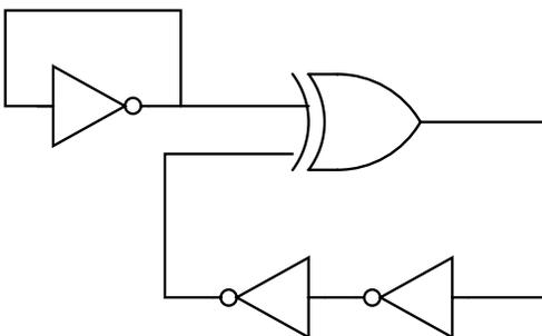
Figure 1.6: Example of Boolean chaos circuit, which consists of one NAND gate with three NOT gates.
