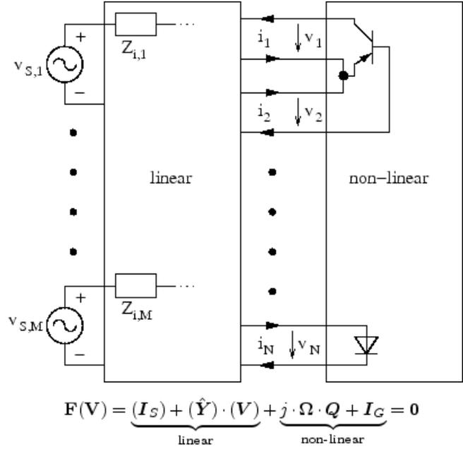
Figure 3.3: Schematic diagram explaining how the harmonic balance simulation operates.  $F(V)$  solves the nonlinear and linear parts separately.  $Y$  is the transadmittance matrix for the linear parts, and  $Q$  and  $I_G$  are the frequency-domain factors for the nonlinear circuits.
