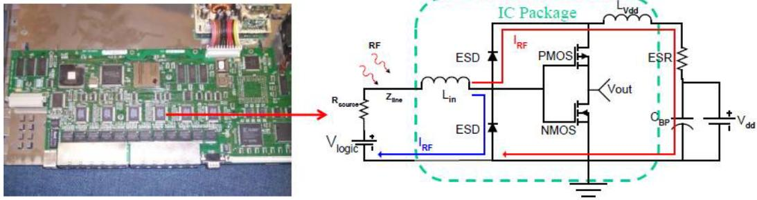
Figure 2.1: Schematic diagram and basic elements in modern CMOS digital ICs.
