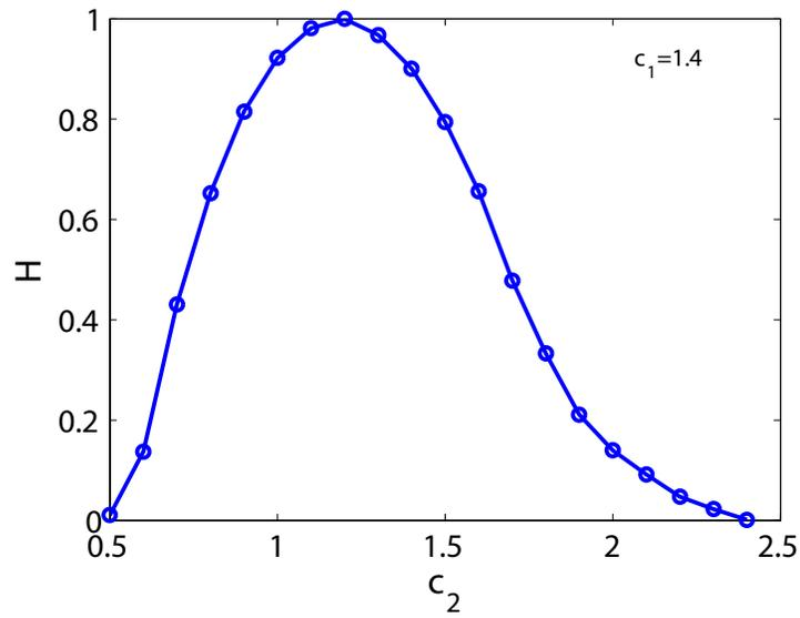
Figure 5.3: Calculated entropy as a function of threshold  $C_2$ . We evaluated the binary sequence of  $C_2 = 1.2$  for statistical properties of random processes using the NIST statistical test.
