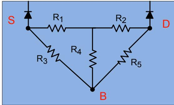
Figure 3.2: Diagram for Berkeley Short-channel IGFET Model 4 substrate resistance network, which models non-quasi static region. This resembles a reverse recovery time of ESD junction diodes during switching.
