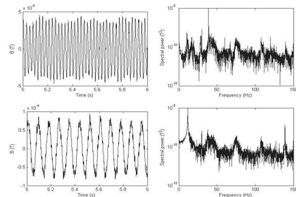
Two time series from a single Hall probe, showing measurements of induction in the presence of a constant, axial magnetic field, along with their power spectra. Experimental parameters are  $(\Omega_i, \Omega_o)/2\pi = (5.7, 29.9)$  Hz, upper;  $(\Omega_i, \Omega_o)/2\pi = (-12.2, 29.9)$  Hz, lower.
