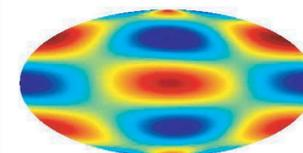
Above: Time series of Gauss coefficients showing a propagating  $g_1$  pattern. Parameters are  $\Omega_i/2\pi = 3.2$  Hz,  $\Omega_o/2\pi = 18$  Hz,  $B_0 = 124$  G, or  $(\chi, S, Rm) = (0.17, 0.84, -105)$ . Left: Snapshot of the magnetic induction on the surface of the sphere, with red indicating outward field and blue indicating inward field. This is the  $(l_{mag}, m, \omega/\Omega_o) = (3, 1, 0.612)$  inertial wave mode (see above).
