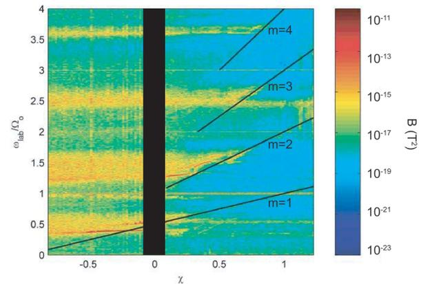
Spectrogram of inner sphere ramp showing oscillatory modes. Normalized rotation rate  $\chi = \Omega_i/\Omega_o$  varies along the horizontal axis, and normalized signal frequency (from an equatorial Hall probe)  $\omega_{lab}/\omega_o$  varies along the vertical. Color indicates power spectral density. Black lines show Mach 2 boundaries; see below. Here  $\Omega_i/2\pi = 29.9$  Hz.
